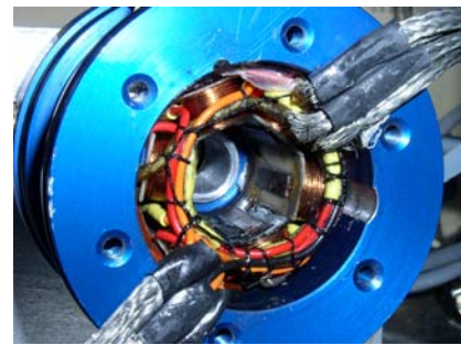
High speed spindle: 140000 rpm
